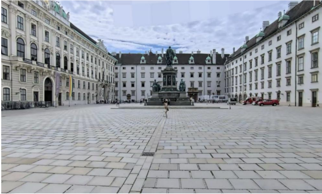
Fig. 2.49 — The square inside the Hofburg Imperial Palace in Vienna, Austria. Use of concealed drainage and pavement surfacing to ensure easy wheelchair access (Apple Maps, n.d.)
