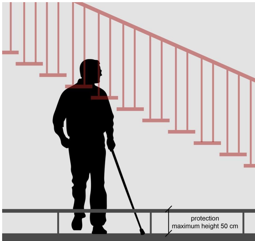
Figure 37. Section diagram illustrating the alternative design proposal of a protection -maximum height 50 cm - detectable by the blind person through the white cane (Authors' work)
