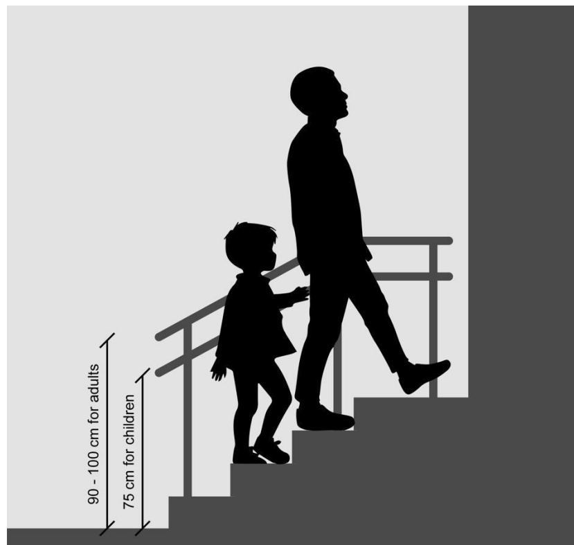
Figure 34. Section diagram illustrating the recommended heights for handrails. (Authors' work)
